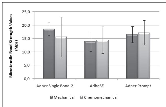
Fig. 2. Microtensile bond strength of the different groups.
